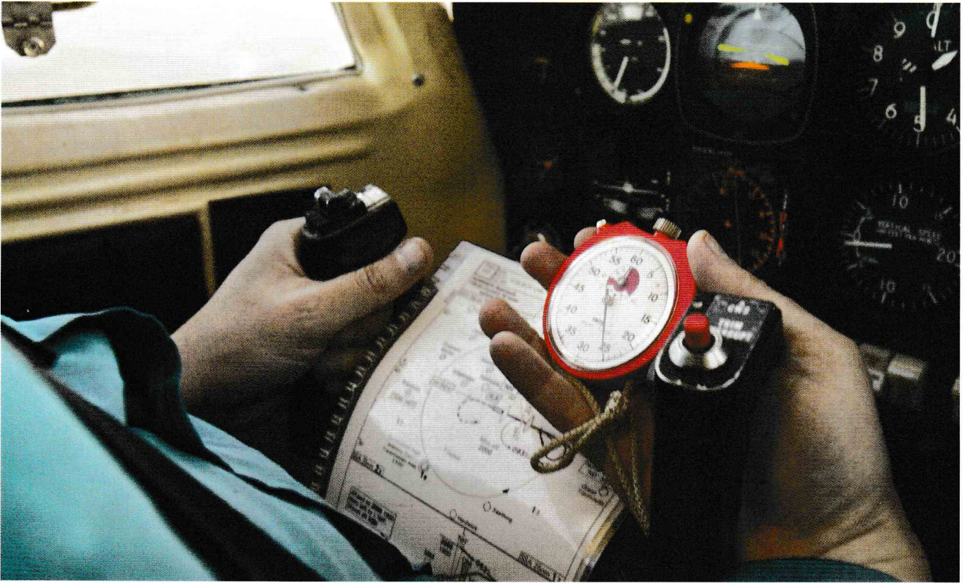
Plate and stopwatch. For procedures without a DME the student is required to use time to assess distance
