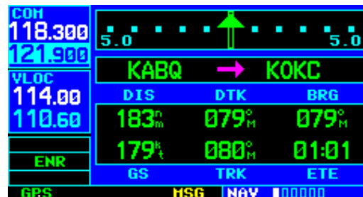
Figure 9-9 GPS Coupled to External CDI
