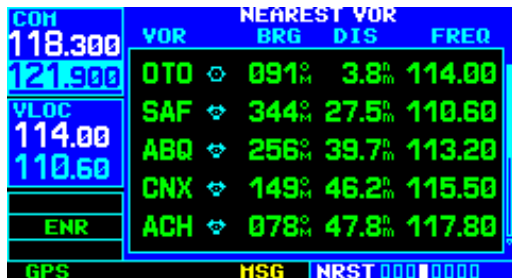
Figure 9-6 Frequency in Standby Field
