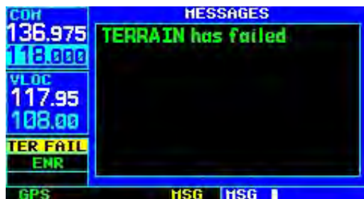
Figure 11-11 'TERRAIN has failed' Message
