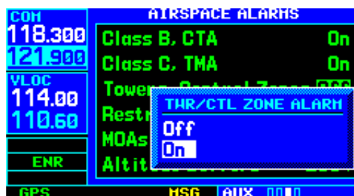
Figure 10-56 TWR/CTL Zone Alarm Window
